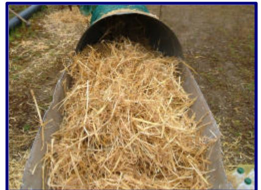
**Step 6:** Take the ramrod and push the straw through the tube and into the netting. One person breaks up the straw and loads it onto the tray. One person pushes it through the machine and the third person guides the sausage out at the end.
